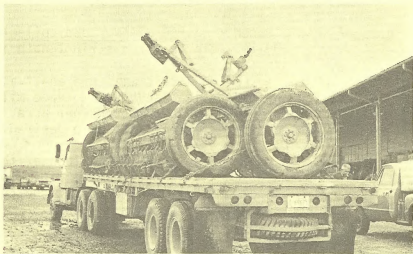
Figure 24. Most highboy trailers will carry four drills.
